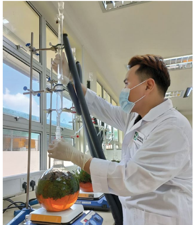
Distillation of essential oil from aromatic plants using the cleverger apparatus
