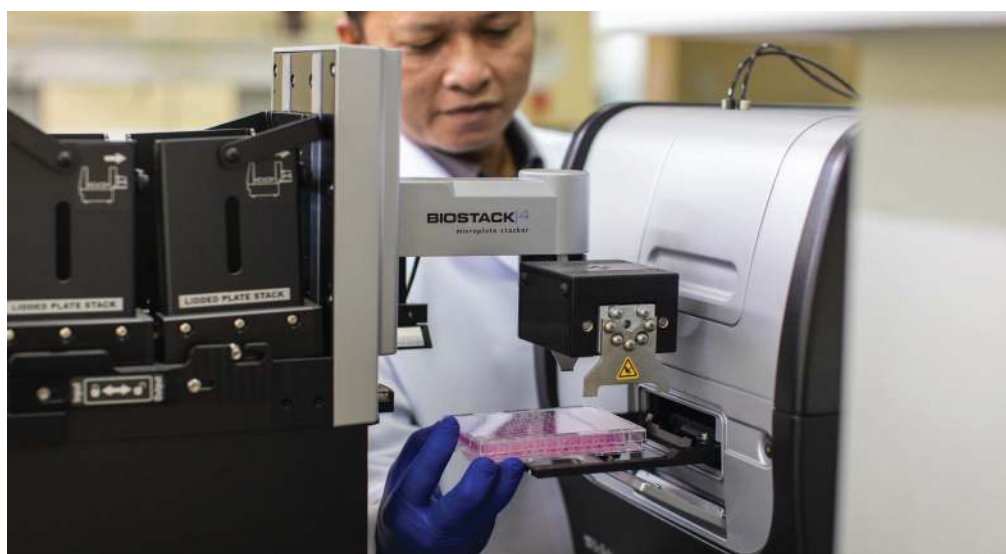
Fluorescence signals measurement with Cytation 3 reader for detection and quantification of target protein.
