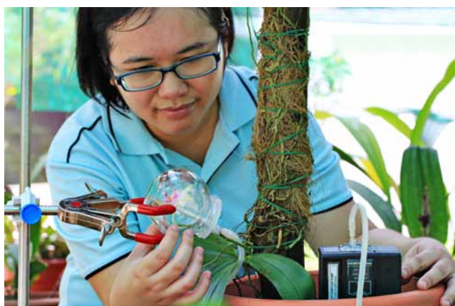
▲ Trapping of Phalaenopsis bellina scent using headspace technique
