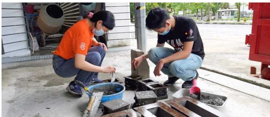
St. Joseph Private School students casting concrete with oil palm shell aggregates.
