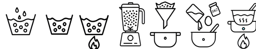
Figure 3: Simplified illustration of the kenaf seed tofu production process
