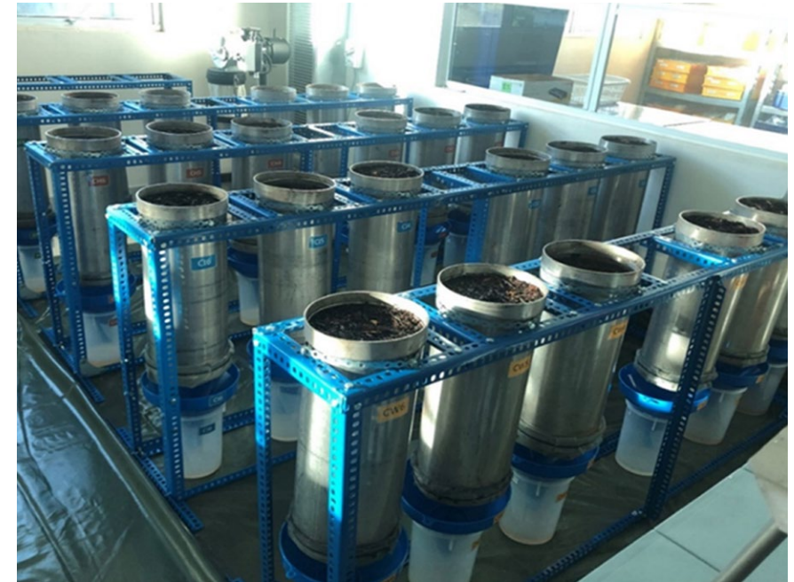
Figure 2: Soil column experimental set-up in the laboratory (Ratai et al., 2025).
