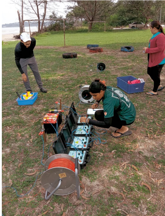
Picture 1: Research team conducting resistivity survey in the field.
