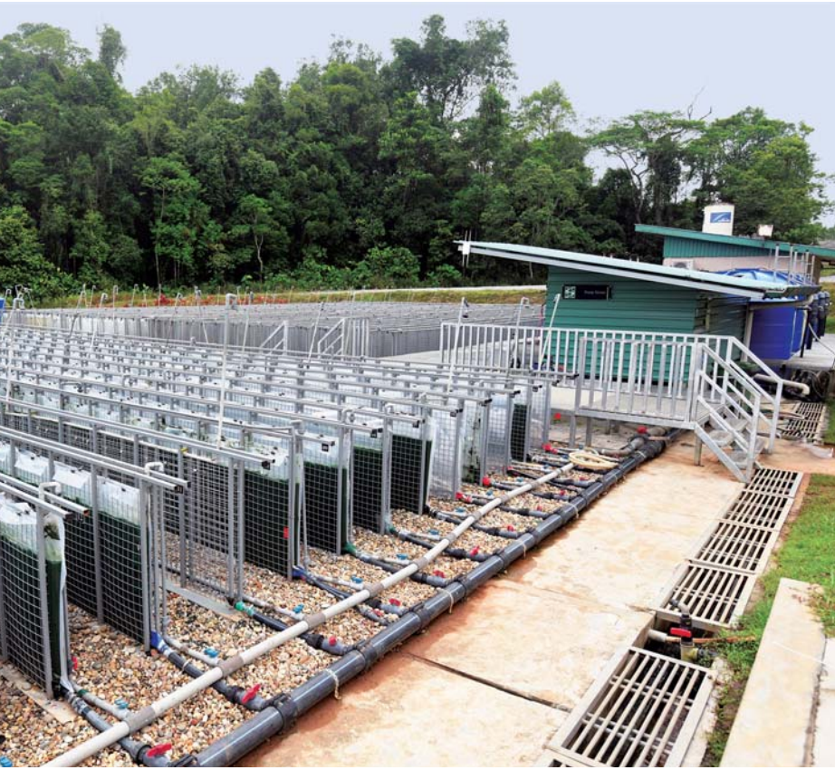
The cost effective flat-panel photo-bioreactor system developed in-house by Sarawak Biodiversity Centre with Mitsubishi Corp and Chitose Laboratory, is built with smart digital monitoring and artificial intelligence for detecting contamination
